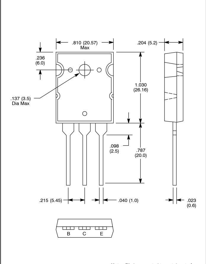
**Note: Pin2** connected to metal part of mounting surface.
