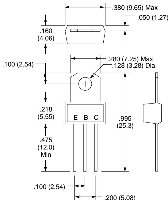
Collector Connected to Tab
