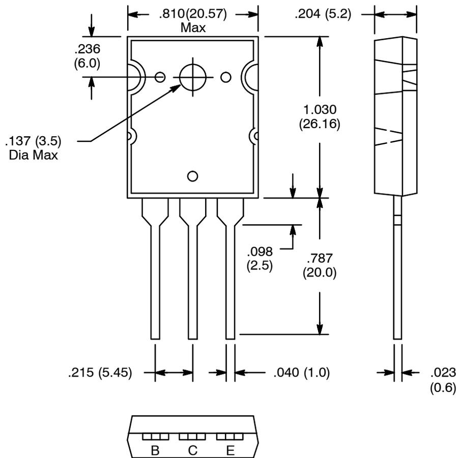
**Note:** Collector connected to heat sink.
