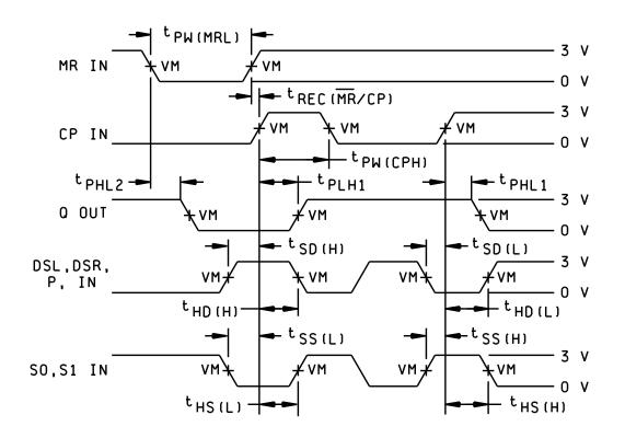
FIGURE 4. Switching time waveforms - Continued.
