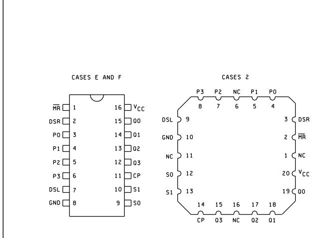
FIGURE 1. Terminal connections.
