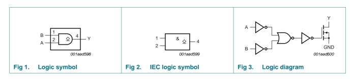
Low-power 2-input AND gate with open-drain
