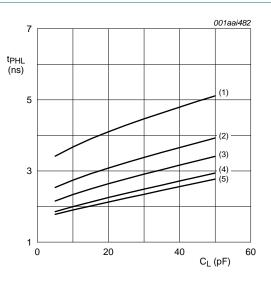
b. HIGH to LOW propagation delay (A to B);  $V_{CC(A)} = 1.8 \text{ V}$
