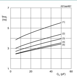
b. HIGH to LOW propagation delay (A to B);  $V_{CC(A)} = 1.2 \text{ V}$
