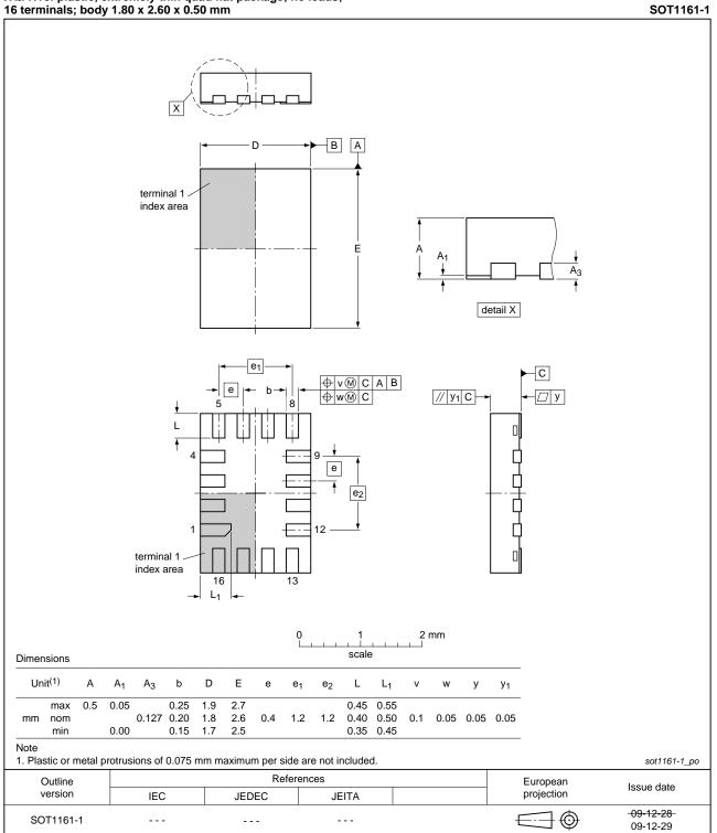
XQFN16: plastic, extremely thin quad flat package; no leads; 16 terminals; body 1.80 x 2.60 x 0.50 mm
