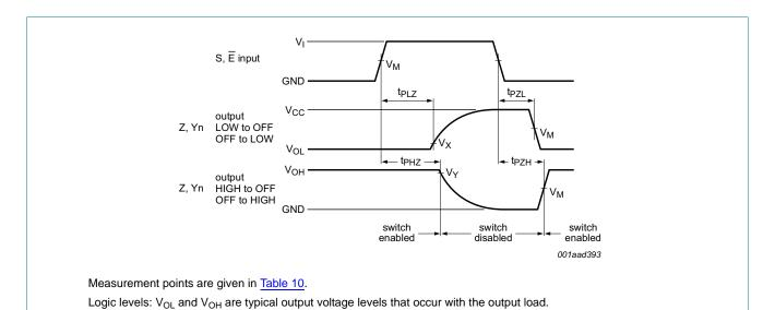
Fig 17. Enable and disable times
