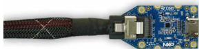
Figure 4: Mini-SAS cable connected to the mini-SAS connector (J5) on the MIPI-DSI to HDMI accessory board.
