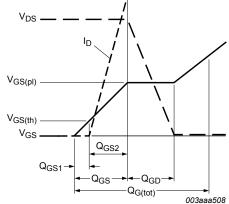
Fig. 14. Gate charge waveform definitions
