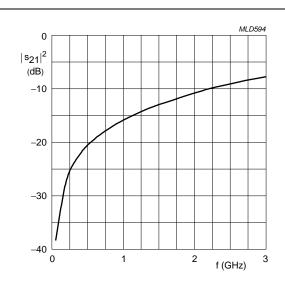
Diode zero biased and inserted in series with a 50  $\Omega$  stripline circuit.  $\rm T_{amb}$  = 25  $^{\circ}\rm C.$
