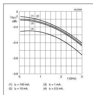
Diode inserted in series with a 50  $\Omega$  stripline circuit and biased via the analyzer Tee network.
