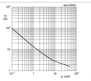
$f = 100 \text{ MHz}; T_i = 25 ^{\circ}\text{C}.$
