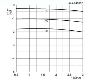
Diode inserted in series with a 50  $\Omega$  stripline circuit and biased via the analyzer T-network;  $T_{amb}$  = 25  $^{\circ}C$
