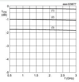
Diode inserted in series with a 50  $\Omega$  strip line circuit and biased via the analyzer T-network. T<sub>amb</sub> = 25  $^{\circ}C.$
