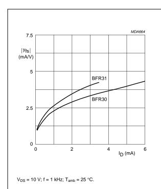
Fig.11 Common source transfer admittance as a function of drain current; typical values.
