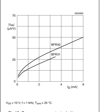
Fig.12 Common source output admittance as a function of drain current; typical values.
