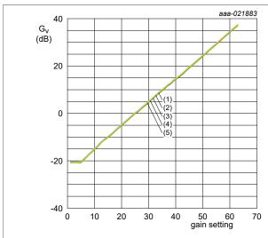
V<sub>CC</sub> = 5 V; current setting = 3; T<sub>amb</sub> = 25 °C
