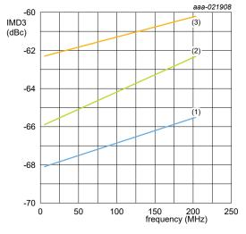
$V_{CC}$  = 5 V; decimal current setting = 3;  $T_{amb}$  = 25 °C;  $P_L$  per tone = 65 dBmV,  $P_i$  per tone = 28 dBmV; 1 MHz tone space; Fix  $P_i$  at 65 dBmV,  $P_o$  / tone = > lower gain setting
