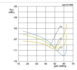
$V_{CC}$  = 5 V; decimal current setting = 3;  $T_{amb}$  = 25 °C;  $P_L$  = 68 dBmV;  $P_i$  = 31 dBmV, Fix Pin at 68 dBmV,  $P_o$  = > lower gain setting
