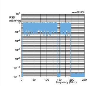
OFDM input signal for ACLR measurement total bandwidth = 192 MHz exclusion band = 147.5 MHz all with a bandwidth of 9.6 MHz.
