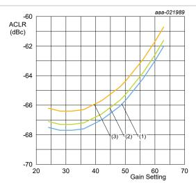
V<sub>CC</sub> = 5 V; decimal current setting = 3; T<sub>amb</sub> = 25 °C Up to decimal gain setting = 60; P<sub>i</sub> = 31 dBmV At decimal gain settings = 61, 62, and 63; P<sub>o</sub> = 68 dBmV Input signal applied as listed in Figure 22
