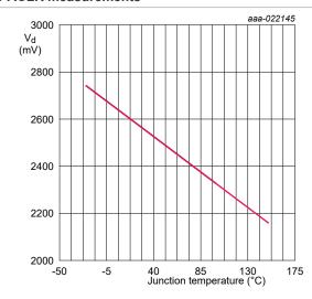
V<sub>CC</sub> = 5 V; decimal current setting = 3 TMP SENS; DC current = 1 mA decimal gain setting = 63
