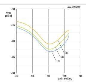
V<sub>CC</sub> = 5 V; decimal current setting = 3; T<sub>amb</sub> = 25 °C; P<sub>L</sub> = 68 dBmV; P<sub>i</sub> = 31 dBmV, Fix P<sub>i</sub> at 68 dBmV, P<sub>o</sub> = > lower gain setting
