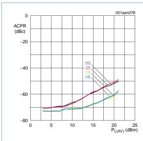
2-carrier W-CDMA; each carrier according to 3GPP test model 1; 64 DPCH; PAR for composite signal = 7.5 dB; 5 MHz carrier spacing.
