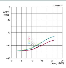
2-carrier W-CDMA; each carrier according to 3GPP test model 1; 64 DPCH; PAR for composite signal = 9 dB; 10 MHz carrier spacing.
