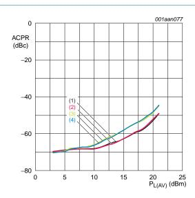
2-carrier W-CDMA; each carrier according to 3GPP test model 1; 64 DPCH; PAR for composite signal = 9 dB; 10 MHz carrier spacing.
