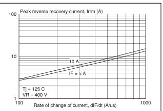
Fig.8. Typical peak reverse recovery current,  $I_{rrm}$  as a function of rate of change of current  $dI_F/dt$ .
