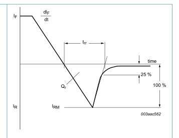
Fig. 6. Reverse recovery definitions; ramp recovery
