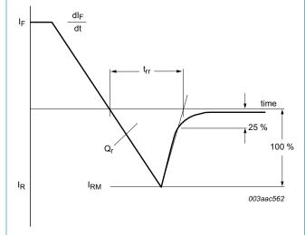
Fig. 5. Reverse recovery definitions; ramp recovery
