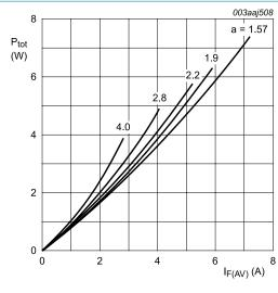
a = form factor =  $I_{F(RMS)}/I_{F(AV)}$  $V_o$  = 0.791 V;  $R_s$  = 0.013  $\Omega$
