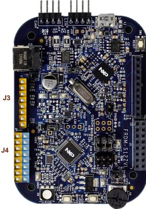
Arduino Compatibility The internal rows of the I/O headers on the DEVKIT-ZVL128 are arranged to fulfill Arduino<sup>™</sup> shields compatibility .
