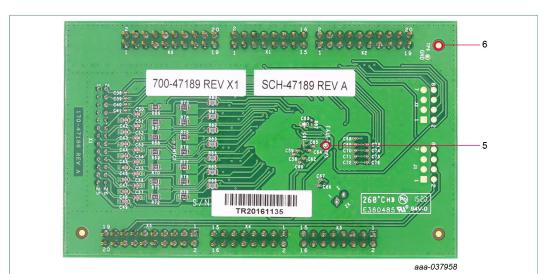
Figure 5. Test points (board bottom)
