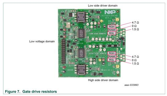
• RAMC - series resistor between IGBT gate and AMC input pin of the GD3100 highside/low-side driver for gate sensing and Active Miller clamping.
