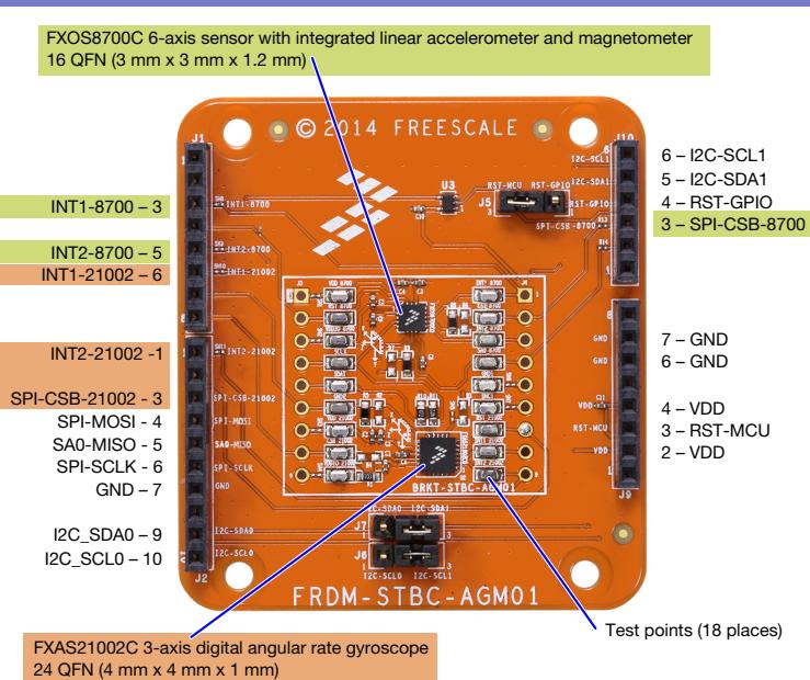
The diagram shows the FRDM-STBC-AGM01 development board with various component labels and connection points:
