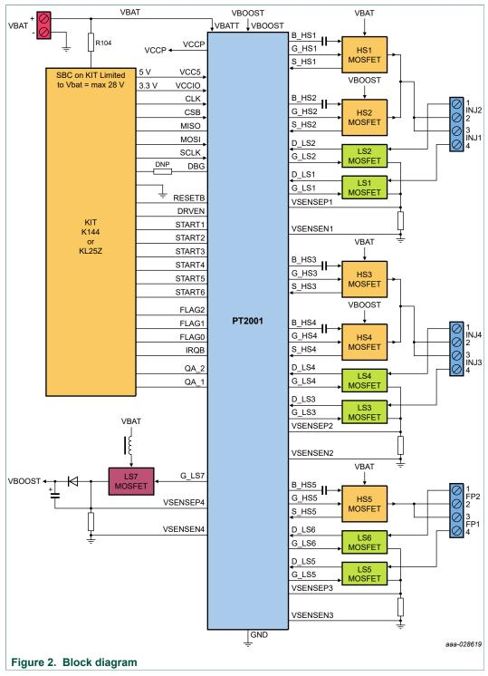
**Note:** The PT2001 supports up to 72 V on the battery line, but the SBC UJA1169 on S32K144 kit only supports 40 V as maximum rating and 28 V full performance. Therefore, the board supply should be limited to 28 V or the MCU kit should be supplied externally (R104 resistor to be removed in this case).
