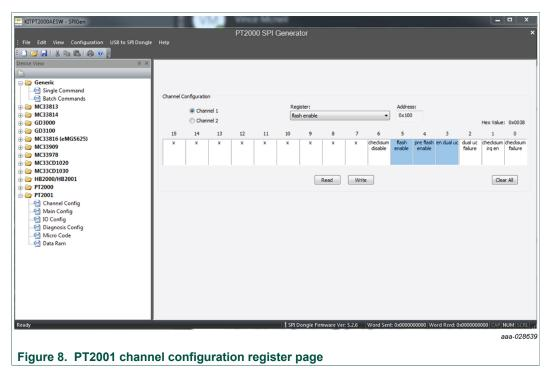
To read or write a specific register on the PT2001, select the register name from the **Register** drop-down on the top center of the page. The register address will be shown to the right of the name. To read the contents of the register, click **Read**. The bits that are set (1) are colored blue; the bits that are cleared (0) are colored white.
