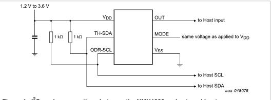
Figure 1. I<sup>2</sup>C mode, connections between the NMH1000 and external host
