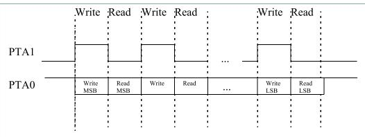
Figure 2. Description of the physical layer on the FXTH87xx22 Simulated SPI interface
