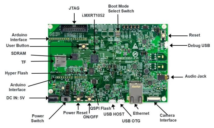
Figure 2. Overview of the MIMXRT1050 EVK Board (Front side)
