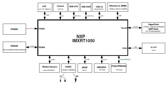
Figure 1. Block diagram
