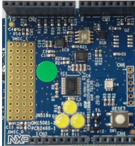
Figure 8 Lighting expansion board
