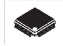
AE SUFFIX (PB-FREE) 98ASA00173D 48-PIN LQFP-EP
