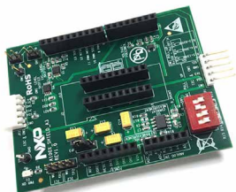
OMA100X-SHLD-EVB Orderable part number: OMA100X-SHLD-EVB An Arduino Uno R3 Interface board
