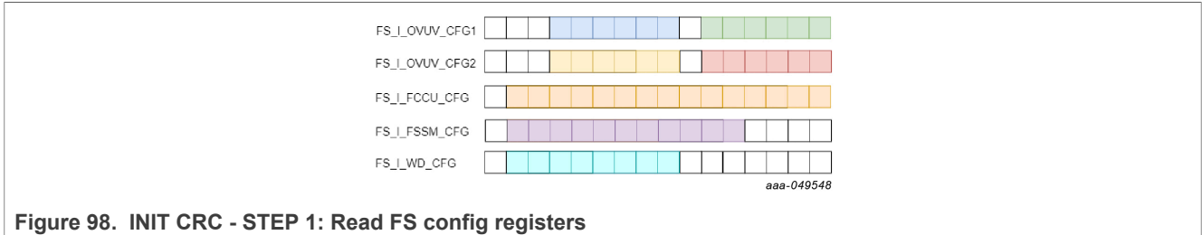
Figure 98. INIT CRC - STEP 1: Read FS config registers
