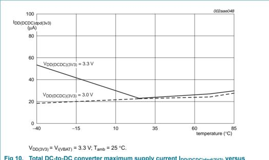
Fig 10. Total DC-to-DC converter maximum supply current I<sub>DD(DCDC)dpd(3V3)</sub> versus temperature in Deep power-down mode
