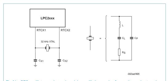
Fig 31. RTC oscillator modes and models: oscillation mode of operation and external crystal model used for  $C_{X1}/C_{X2}$  evaluation
