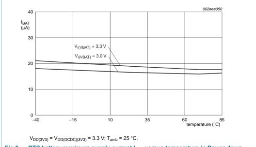
RTC battery maximum supply current  $I_{BAT}$  versus temperature in Power-down Fig 6. mode
