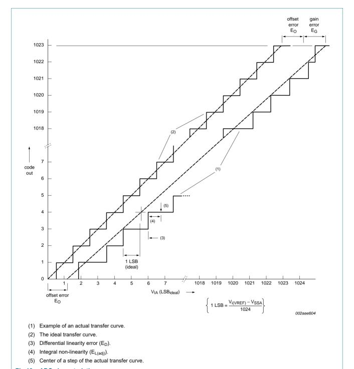
Fig 19. ADC characteristics
