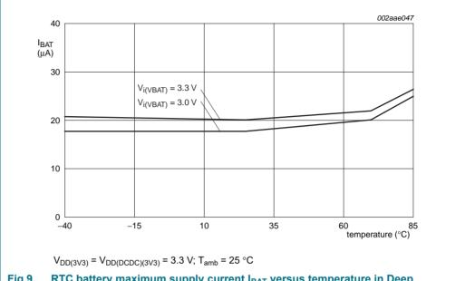
Fig 9. RTC battery maximum supply current I<sub>BAT</sub> versus temperature in Deep power-down mode
