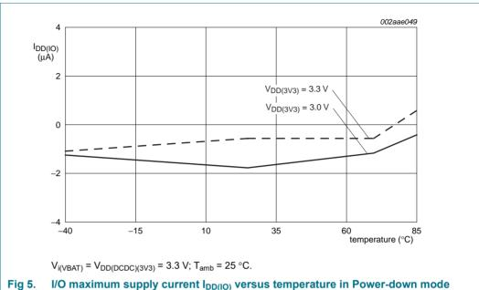
I/O maximum supply current  $I_{\text{DD(IO)}}$  versus temperature in Power-down mode
