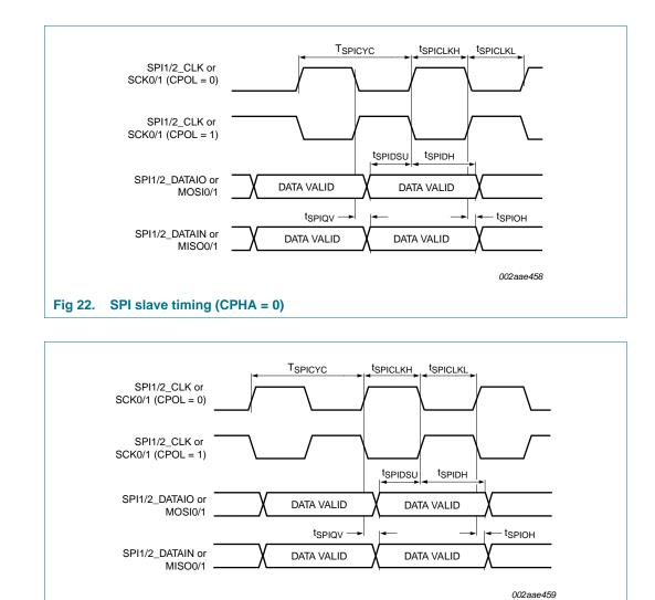
Fig 23. SPI slave timing (CPHA = 1)
