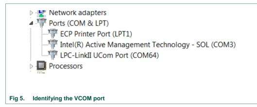
If the J-Link firmware image has been programmed into the Debug Probe and DFU boot mode is not being used, then a VCOM device called Jlink CDC UART port will appear instead of the LPC-LinkII UCom port.
