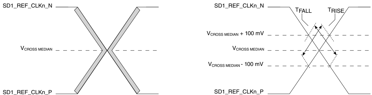
Figure 78. Single-ended measurement points for rise and fall time matching
