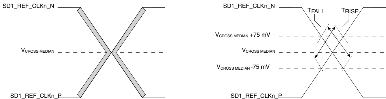
Figure 93. Single-ended measurement points for rise and fall time matching
