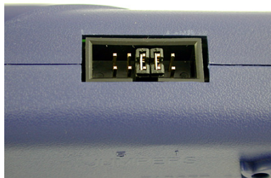
Figure 3-15: Jumper Settings for Target Power Connection via Cyclone PRO Board Power and Power Out Jack of Cyclone PRO
