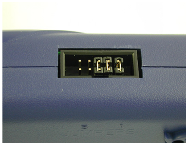
Figure 3-17: Jumper Settings for Target Power Connection via Cyclone PRO Board Power and Pin 15 of Cyclone PRO MON08 Connector
