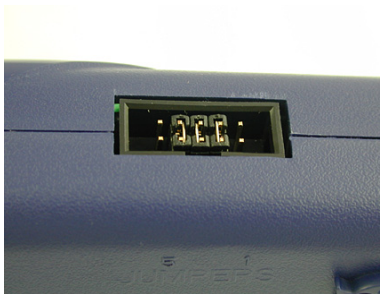
Figure 3-19: Jumper Settings for Target Power Connection via Cyclone PRO Board Power and Pin 6 of Cyclone PRO BDM Connector
