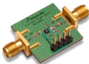
Figure 12. Typical Assembled Evaluation Board with SMA Connectors
