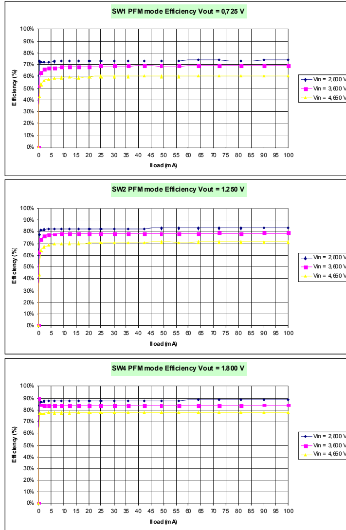
Figure 17. Buck Regulator PFM Efficiency
