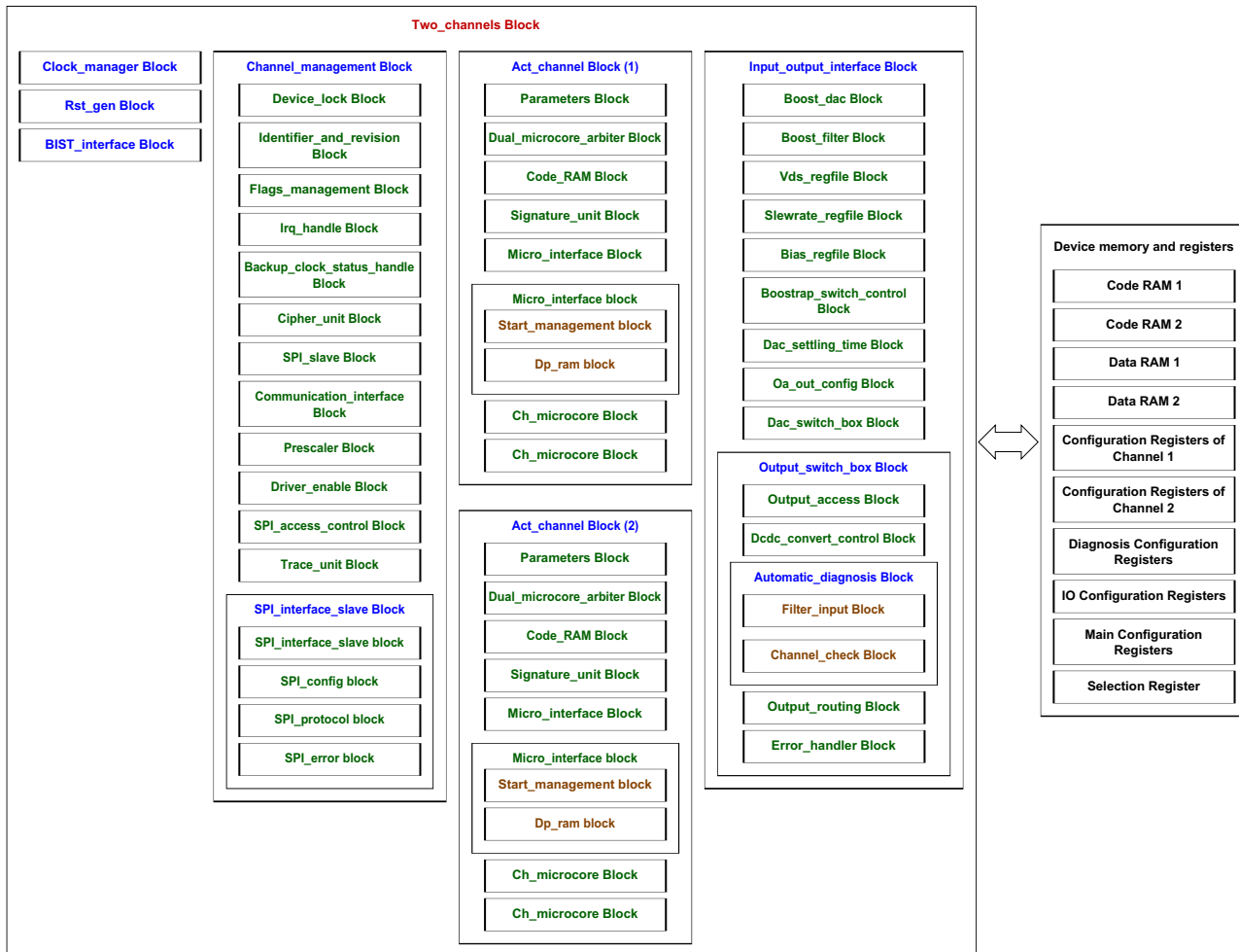
Figure 24. Device logic block hierarchic overview
