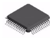
AE SUFFIX (PB-FREE) 98ASA00173D 48-PIN LQFP-EP
