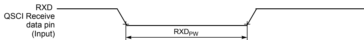
Figure 10-12 RXD Pulse Width
