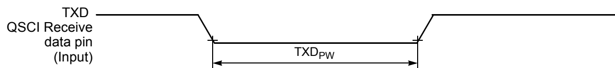
Figure 10-13 TXD Pulse Width
