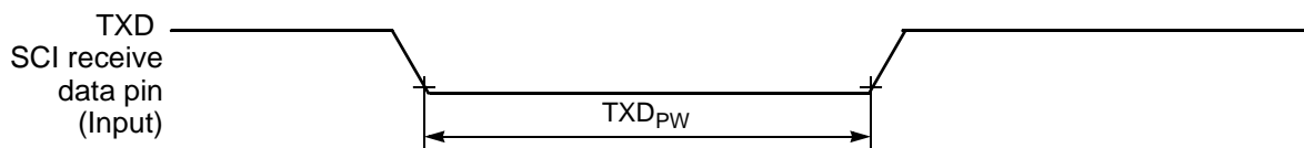
Figure 10-16 TXD Pulse Width
