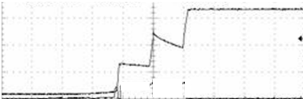
Figure 22. Supply Voltage Drop
