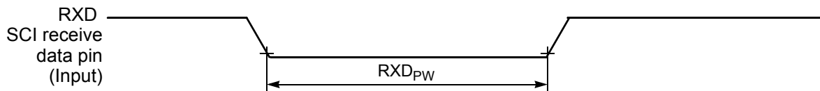
Figure 10-16 RXD Pulse Width
