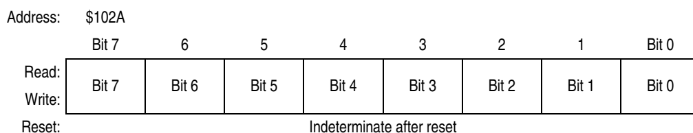
Figure 8-5. Serial Peripheral Data I/O Register (SPDR)
