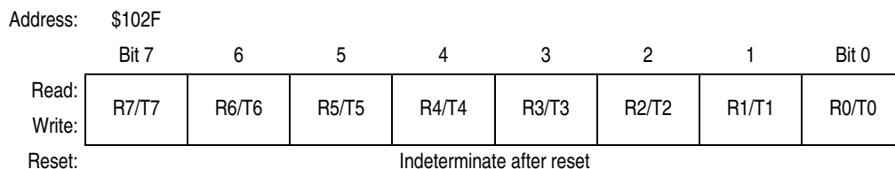
Figure 7-3. Serial Communications Data Register (SCDR)
