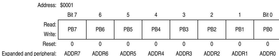
Figure 6-3. Port B Data Register (PORTB)
