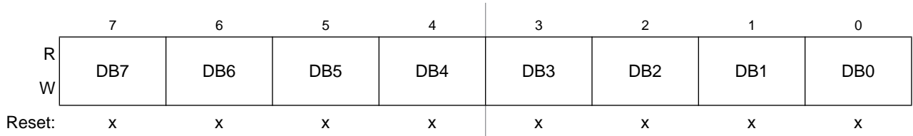
Figure 12-33. Data Segment Registers (DSR0–DSR7) — Extended Identifier Mapping
