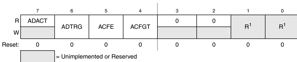
Figure 9-5. Status and Control Register 2 (ADCSC2)
