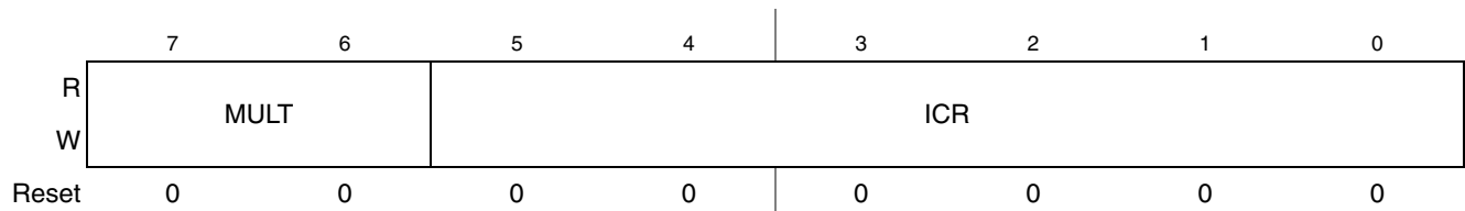
Figure 11-4. IIC Frequency Divider Register (IICF)
