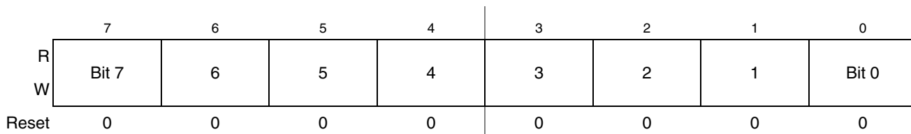
Figure 16-14. TPM Channel Value Register Low (TPMxCnVL)
