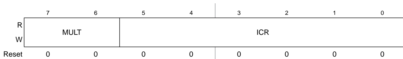
Figure 11-4. IIC Frequency Divider Register (IICF)
